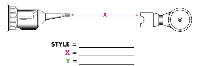
X measurement will be from the tip of the output shaft to the center line of the universal joint or flat of the flange on most all 2wd vehicles. Y measurement will be how far the output shaft protrudes from the seal.
